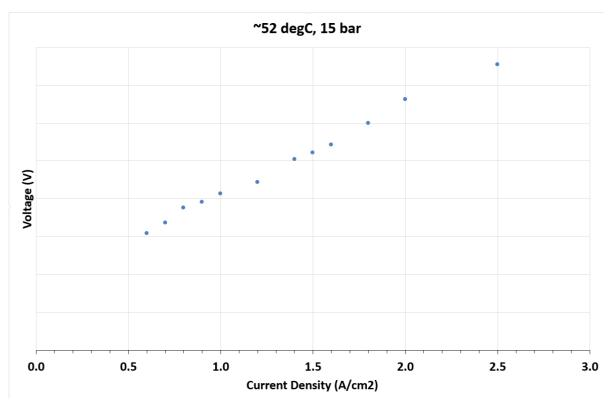
System I – V curve showing plant operation during FAT. Due to the public nature of this report the Voltage figures have been removed for confidentiality reasons.
